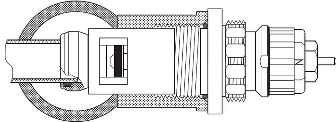
Integrated valves, type RA-N (013G1382) and RA-U (013G1383), with built-in presetting are designed for incorporation into valve radiators from different radiator manufacturers.
