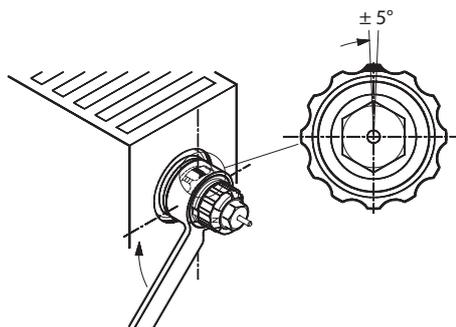
Installation of an integrated valve at radiator manufacturer's plant
